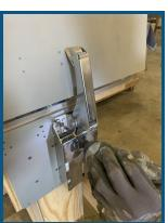
closed. Then secure the hardware (with the front cover removed) to the mounting plate.
