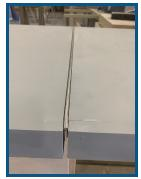
If the piano hinge is properly placed, the hardware can now be secured to the die wall. Most flip gates require either two or three sets of hardware, based on their size. There is a plate provided to mount the hardware if the die wall is not wide enough to accommodate it. If needed, screw the mounting plate into the die wall. The top of the mounting plate should be just below the bottom of the flip gate when
